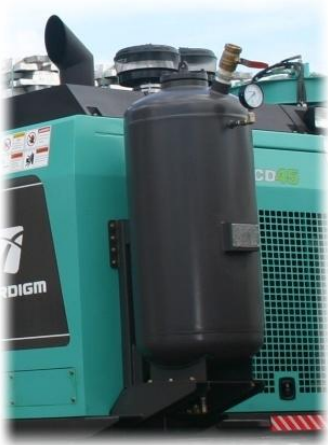
- Water injection system
